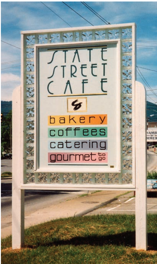
Hand lettered and airbrushed on 4-by-6-ft. overlaid plywood panel finished with Chromatic® enamel [1Shot, 219-949-1684, www.1shot.com]. The framed glass block is attached to 4-by-4-in. posts.
