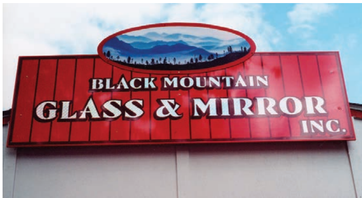
"Cracked ice" holographic film [Graphic Films, Inc., 800-634-7523, www.fdcfilms.com] panels on 3-by-8-ft. AlumaCorr™ panel with plastic trim. The graphic is hand painted and airbrushed on Fiber Brite™ [US Highway Products, 800-883-8363, www.fiberbrite.com] board, clear coated with Frog Juice [Far from Normal Supply, 800-877-1907].
