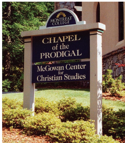
Vinyl film on 18-by-42-in. aluminum panel finished with two-part urethane [Akzo Nobel Coatings, 770-662-8464, www.signfinishes.com ]. The header was sandblasted in redwood then cast in resin by Goldenwest Manufacturing [530-272-1133].
